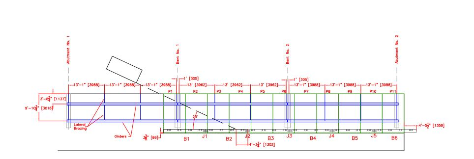
Notes: (1) FRP deck panels are to be installed starting with panel no. 11 (P11) and ending with panel no. 1 (P1).
